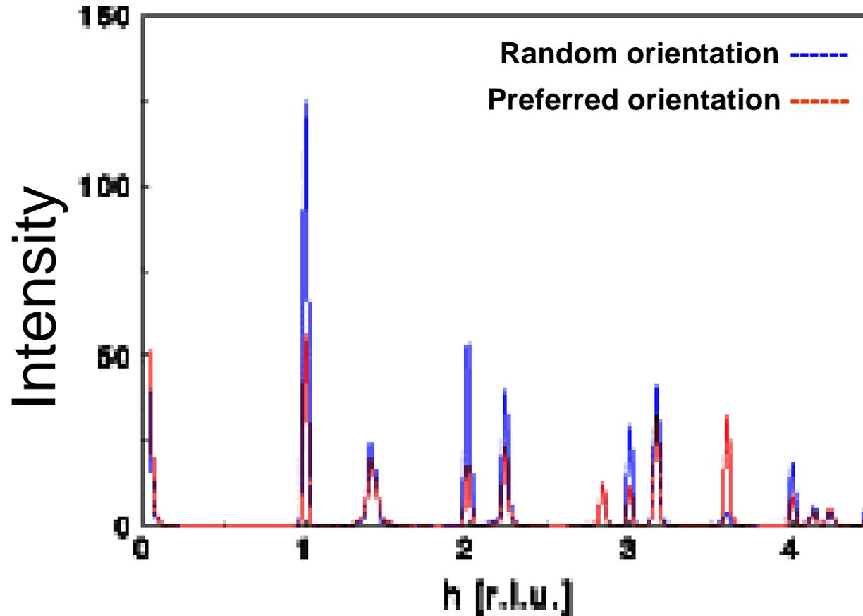
It is noted that due to preferred orientation several blue peaks are completely missing and the intensity of other blue peaks is very misleading. Preferred orientation can substantially alter the appearance of the powder pattern. It is a serious problem in experimental powder diffraction.
