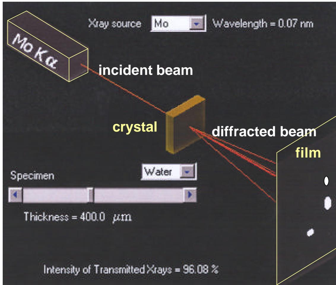
Effect of sample thickness on the absorption of X-rays
