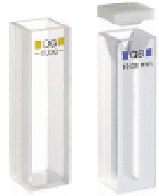
The cells are often designed so that the light beam travels a distance of **1 cm** through the contents (1 mm for low volume).
