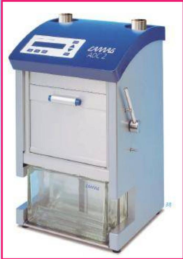
In ADC2 chromatogram development is fully automatic and reproducible, independent of environmental effects. The activity and pre-conditioning of the layer, chamber saturation, developing distance and final drying can be pre-set and automatically monitored by the ADC2. Two modes of operation are possible: stand-alone with input of parameters via keypad or remote operation from winCATS with process monitoring, documentation of operating parameters and reporting.
