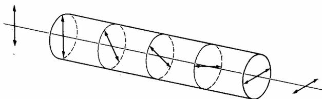
Figure 3: Rotation of polarized light plane by a sample with an optical active substance and the influence of the length of sample tube
