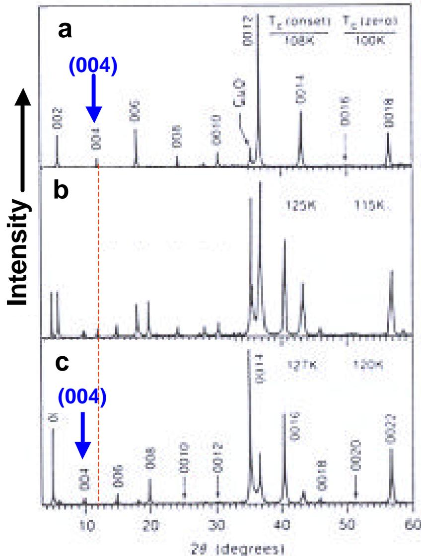
Diffraction patterns of three Superconducting thin films annealed for different times.
