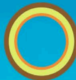
Capillary Wall Coated Open Tubular (WCOT)
