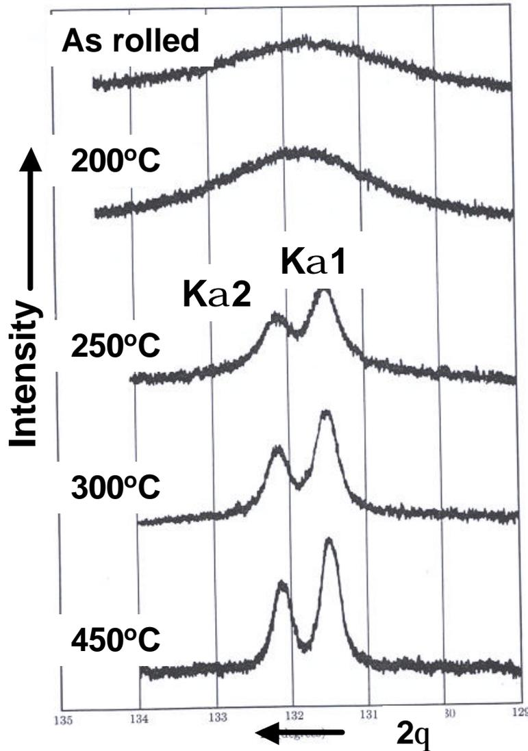
(331) Peak of cold-rolled and Annealed 70Cu-30Zn (brass)
