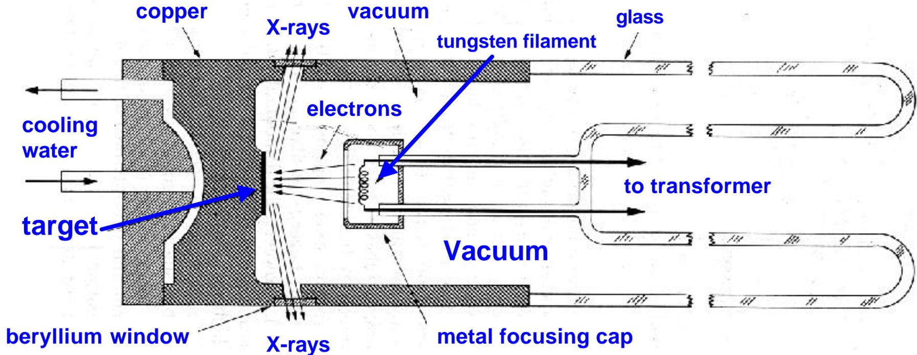
X-rays are produced whenever high-speed electrons collide with a metal target. A source of electrons – hot W filament, a high accelerating voltage between the cathode (W) and the anode and a metal target, Cu, Al, Mo, Mg. The anode is a water-cooled block of Cu containing desired target metal.
