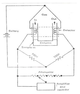
Fig.11 – Thermal conductivity detector.
