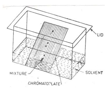
Fig.6- Apparatus for Thin layer chromatography
