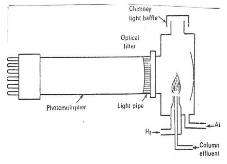
Fig.10- Flame photometric detector.
