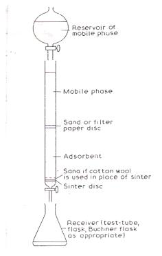
Fig.8- Apparatus for column chromatography.
